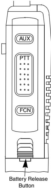
**AUX (Auxiliary)** - This is a dealer programmable switch that can control various functions (see page 9). With the limited keypad (3-key) version, it is also the CLR key.
