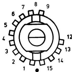
5. Remove the spanner nut and old star washer. Install the new star washer. Make sure that the removed tabs are opposite the numbers to be selected.
