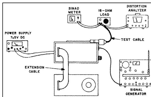
**Figure 8-3 Receiver Test Set-Up**
