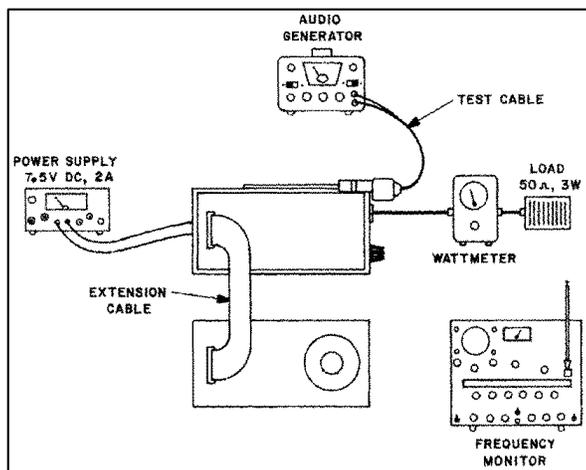
**Figure 8-2 Transmitter Test Set-Up**
