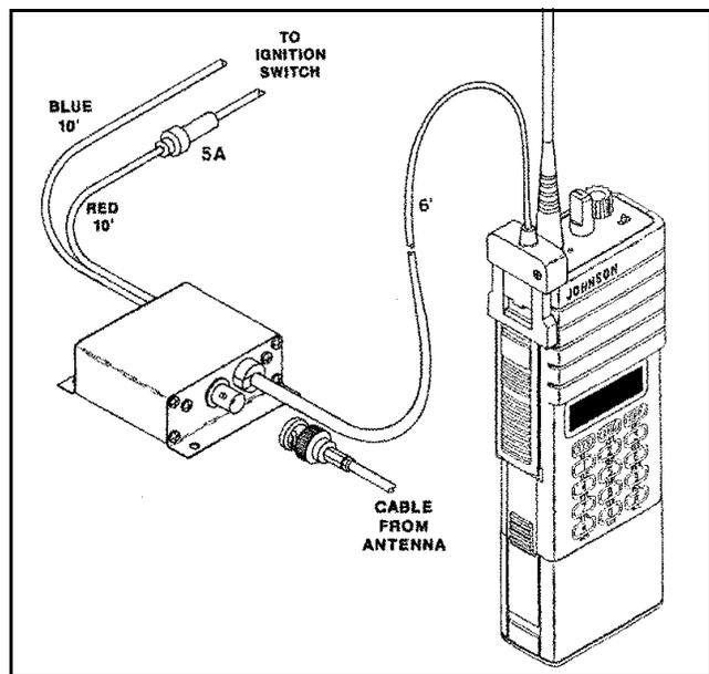
Figure 5-2 Vehicular Charger Components
