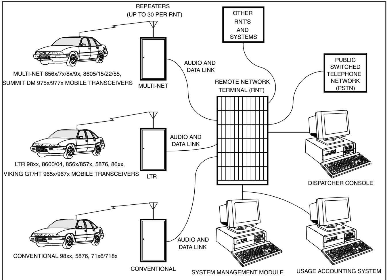
Figure 2-1 Multi-Net System Components
