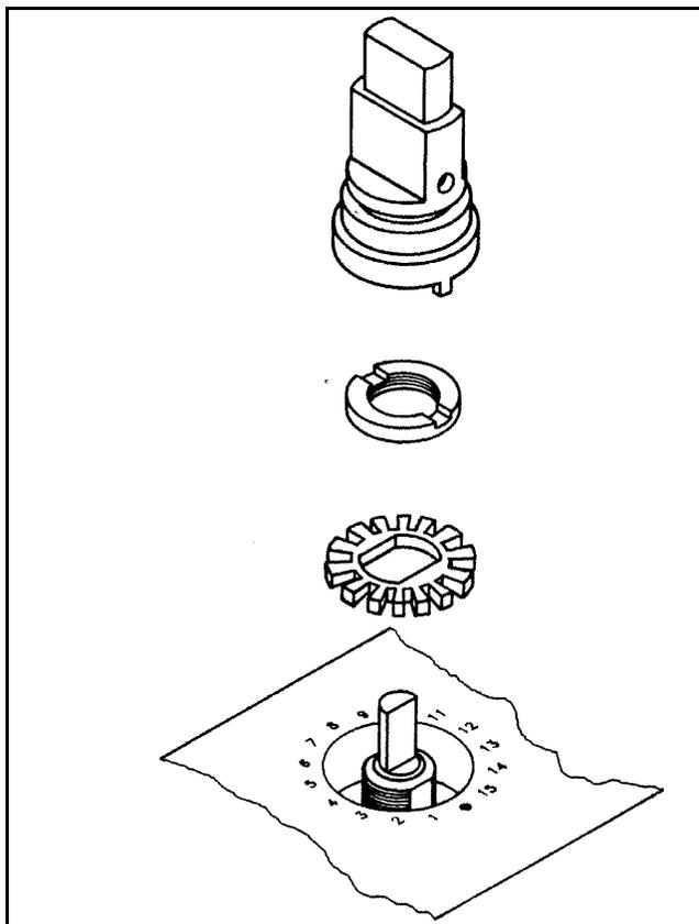
**Figure 1-1 Quick Select Switch Exploded View**
