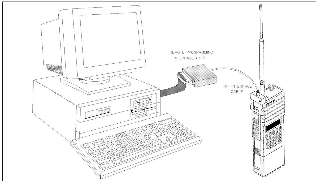
Figure 4-1 Programming Setup
