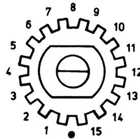
3. The tabs removed are *opposite* the positions to be selected. Therefore, determine what numbers are opposite and then mark the tabs between those numbers. For example, to select positions 1-4, mark the three tabs between 9 and 12.
