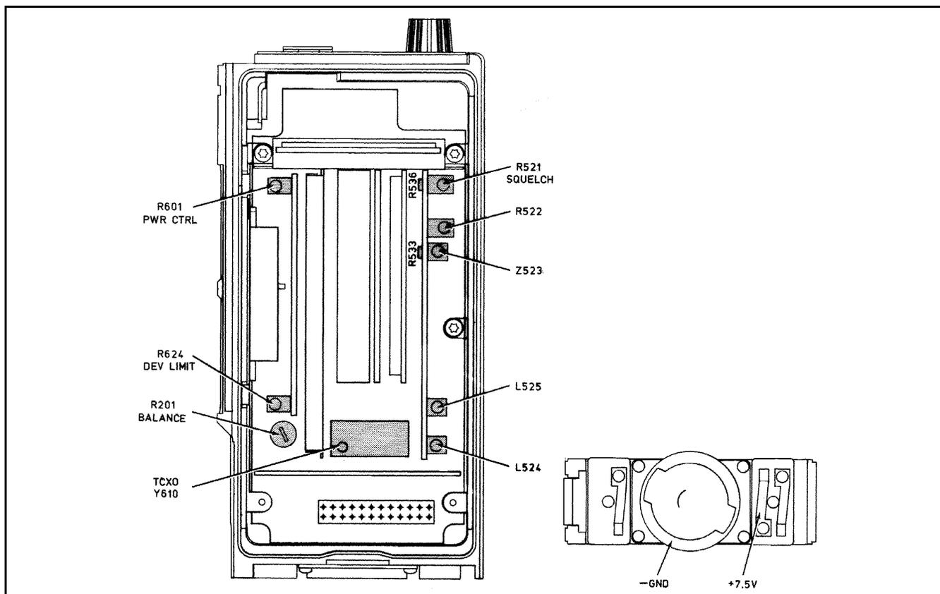
**Figure 8-4 Alignment Points Diagram**
