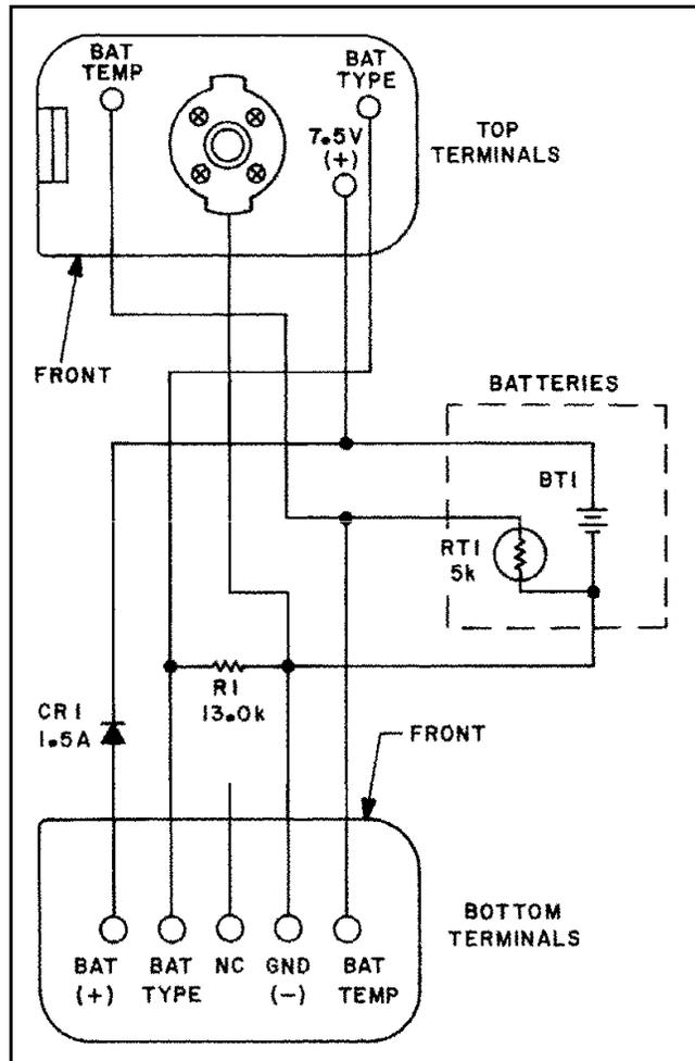
**Figure 5-1 Battery Schematic**
