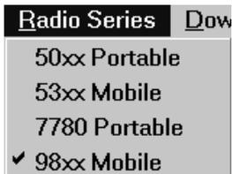
The Radio Series menu show above selects the radio type (9883 Mobile) being programmed.
