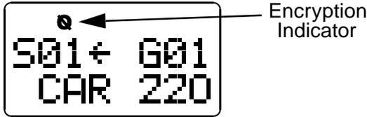
If you have the ENCRYPT menu parameter or ENCPT option switch, the encryption group programming can be temporarily overridden. Selecting another system or group causes encryption to revert to the status programmed for that group.
