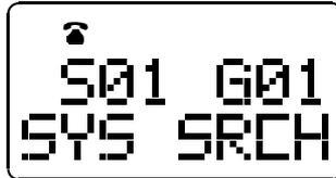
The transceiver then attempts to access, in succession, other systems that have a group programmed for telephone calls. As each system is accessed, a beep sounds. If a system is successfully accessed, the new system/group is selected and a dial tone sounds. The telephone call must then be placed within a few seconds or normal operation resumes. If no system could be accessed, the intercept tone sounds, “NO PHONE” is displayed, the system/group does not change, and the feature deactivates.
