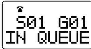
When the radio system becomes available, it is automatically accessed. A beep then sounds and a dial tone is heard. The call can then be placed if desired. The queue mode is exited before the call is placed if any of the following occur (exit is indicated when “IN QUEUE” is no longer displayed).
