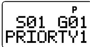
When a message is detected on a first priority group while listening to a non-priority message, a tone sounds, “PRIORITY1” is flashed on the lower line of the display, and the transceiver changes to that system/group to receive the message. Likewise, if a message is received on a second priority group, “PRIORITY2” is displayed. When the priority message is
