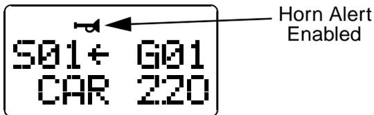
When enabled, the horn alert pulses on and off for 1-8 cycles and then goes back to the disabled state. To change the currently selected horn alert mode, the HORN option switch or HRN ALRT menu parameter can be used if available (see page 30).
