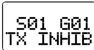
One use of this feature is to prevent the accidental interruption of a call in progress. This could happen when the other party unkeys or if a higher priority ID is transmitted. It may also be used to provide an indication that the mobile you are calling is busy with another call. A similar Transmit Disable On Busy feature is available on conventional systems (see page 44).
