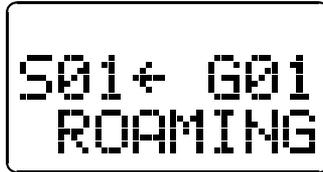
The new system is the first higher system with a different site that could be accessed (wrap-around occurs after the highest system is accessed). The new group is either the same group that was displayed before roaming occurred or the last selected group of that system (programming determines which is selected).
