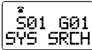
The transceiver then attempts to access, in succession, other systems that have a group programmed for telephone calls. As each system is accessed, a beep sounds. If a system is accessed, the new system/group is selected and a dial tone sounds. The telephone call must then be placed within a few seconds or normal operation resumes. If no system could be accessed, the intercept tone sounds, “NO PHONE” is displayed, the system/group does not change, and the feature deactivates.
