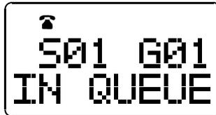
When the radio system becomes available, it is automatically accessed. A beep then sounds and a dial tone is heard. The call can then be placed if desired. The queue mode is exited before the call is placed if any of the following occur (exit is indicated when “IN QUEUE” is no longer displayed).
