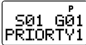
When a message is detected on a first priority group while listening to a non-priority message, a tone sounds, “PRIORITY1” is flashed on the lower line of the display, and the transceiver changes to that system/group to receive the message. Likewise, if a message is received on a second priority group, “PRIORITY2” is displayed. When the priority message is complete, the transceiver returns to the previous system/group. If a message is still present, it is received.
